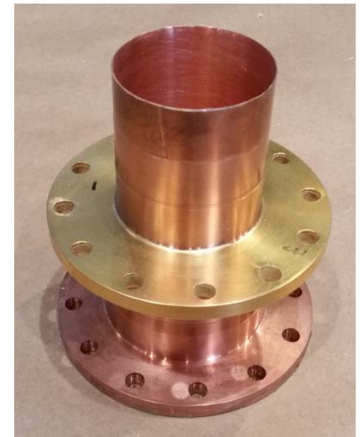
Completed 1-piece copper inj. vol. copper body. Note gold-plated anchor plate (shown upside-down).
