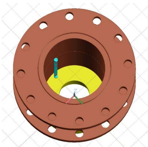
Left: CAD model of the level sensor (light blue) mounted in the injection volume. The small red "dots" are bare ROX sensors. Below: the completed Vespel support rod.
