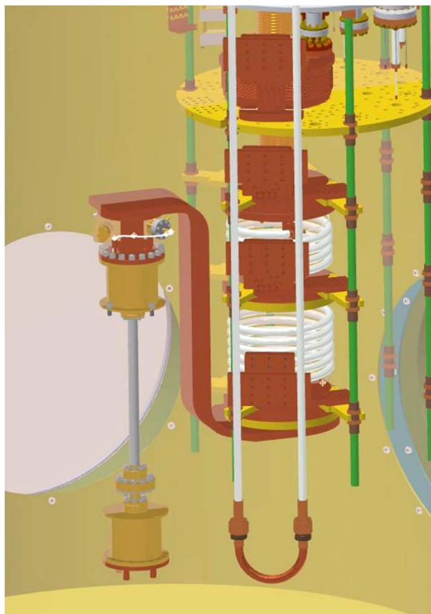
The heat-flush with Nuclepore membrane holder mounted on DR.
