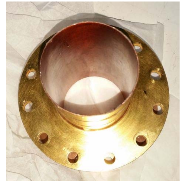
The injection volume body after seamless Kapton tubing was bonded to the inside surface.
