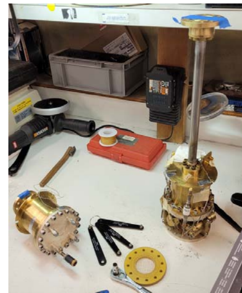
The Harvard heat-flush test hardware disassembled to install Nuclepore membrane
