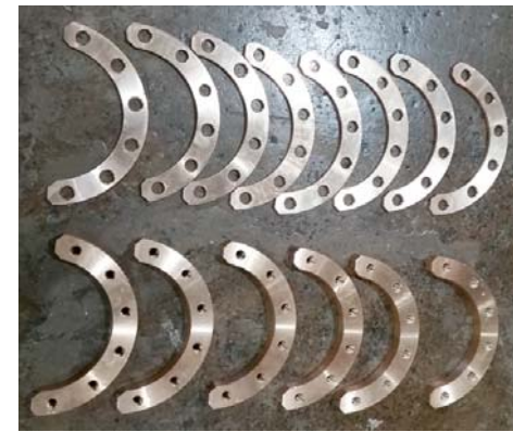
Nut and washer plates used to bolt together soft copper flanges
