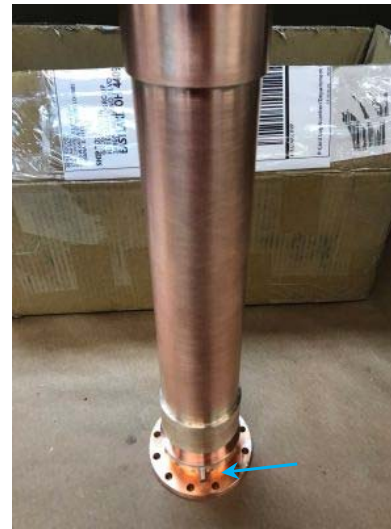
Brazed copper spool piece. This connects the inj. volume to the film burner. Note wiring feed-through bushing for level sensor (see arrow).
