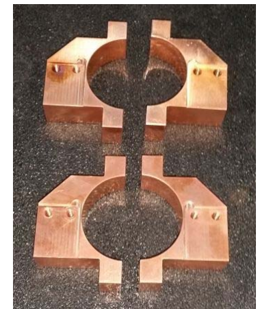
Copper clamps for thermally anchoring the beam line tube to the thermal shields.
