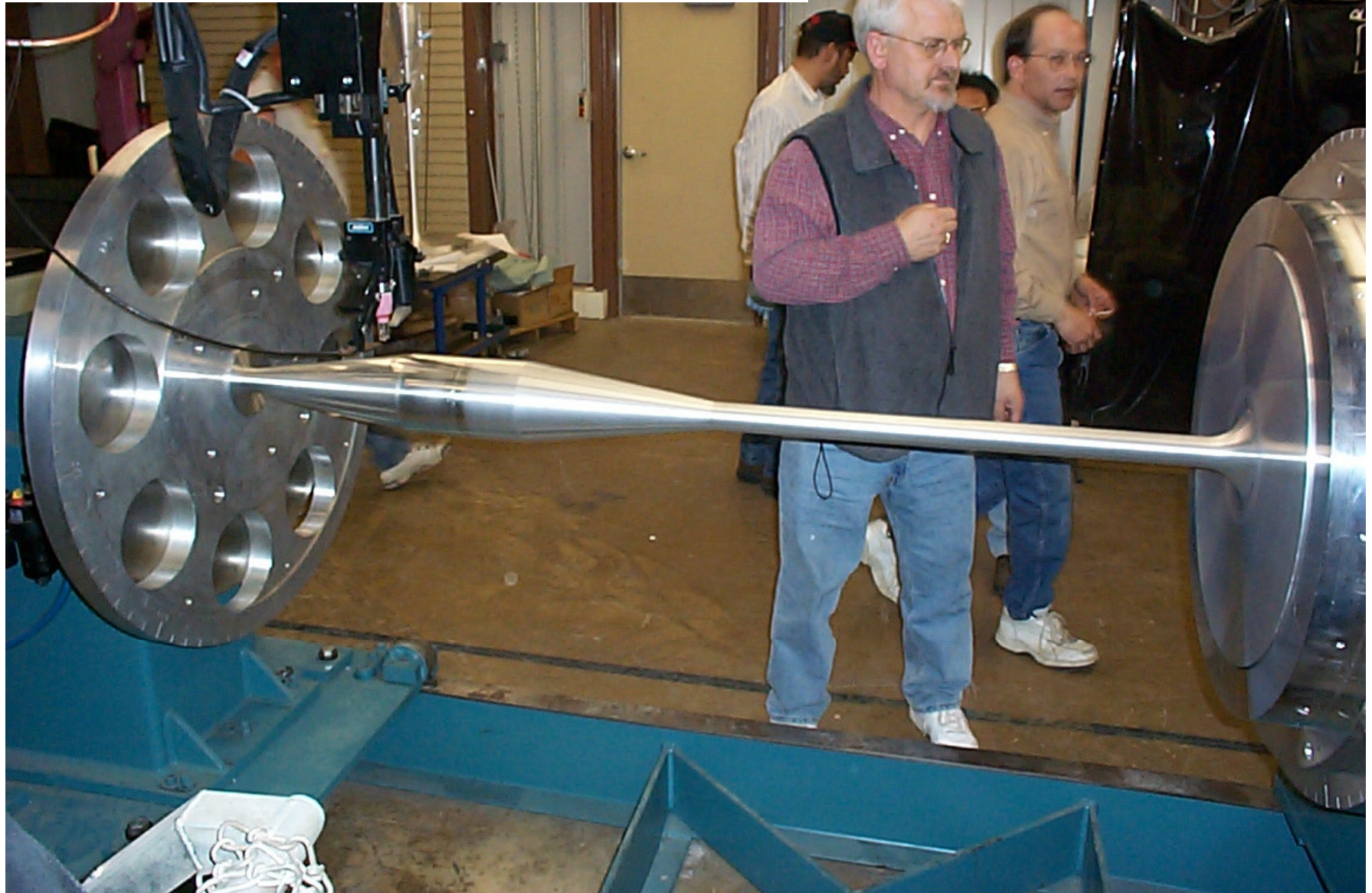
MiniBooNE prototype horn inner conductor on the welding machine
